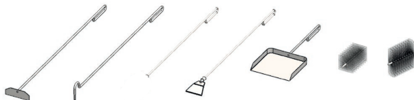
Drawing 10 - Accessories for boiler maintenance and cleaning
